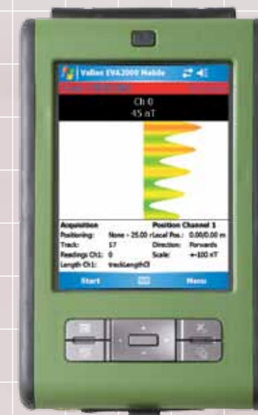
Real-time data monitoring: scrolling curve of survey data
